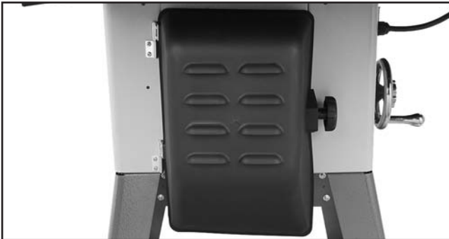
Figure 26. Motor cover installed on saw.
